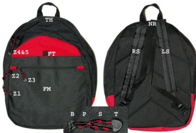
FIG. 1—The regions of a backpack swabbed postdeflagration. Eleven areas of each backpack were targeted for postblast DNA recovery including the five zippers (Z1–Z5), top handle (TH), front tab (FT), front middle region (FM), left strap (LS), right strap (RS), and the neck region (NR). Also shown is an intact zipper with all four components including the base (B), pull (P), string (S), and tab (T). In many instances fewer than 11 targeted regions were recovered.
