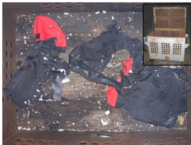
FIG. 2—Exemplary backpack destruction inside the crate following deflagration of a PVC pipe bomb. Backpacks housing steel pipe bombs suffered considerably more fragmentation. The crate (inset), approximately 3 feet wide, was designed to limit the dispersal of IED and backpack fragments. Walls and lid were constructed of steel with holes cut in them to relieve pressure from the blast; the floor was made of wood.
